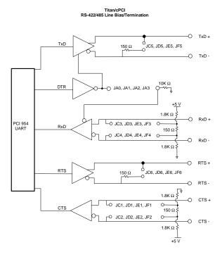
Figure 7: RS-422/485 Partial Schematic
